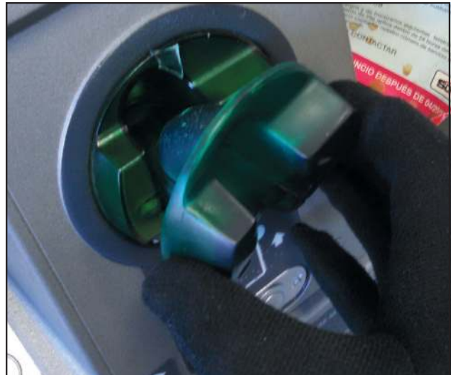
Pictured: the skimming device which was overlaid over the access door of the ATM.
